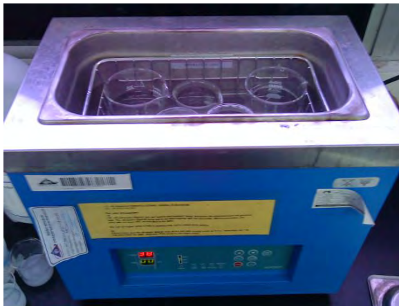
Cleaning process at room temperature using JEIOTECH US-05 Ultrasonic Cleaner (5L).
