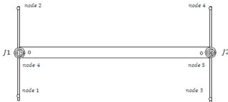
Fig.6: Detailed out cross-section (plan view) of cruciform column for N10 and N14
