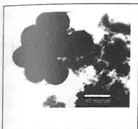
Figure 4. Morphology of BTS3T/TEOS (1:4) by SEM
