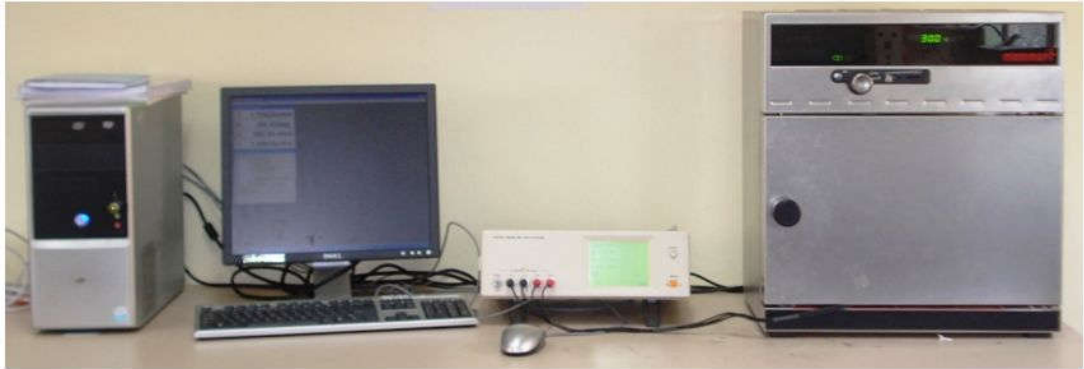
Figure 3.5 The EIS (HIOKI 3532–50 LCR Hi Tester) equipped with a MEMMERT oven and interfaced to a personal computer.
