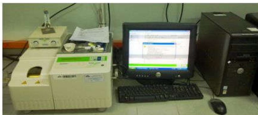
Figure 3.4 The thermogravimetric analyzer used in this study.
