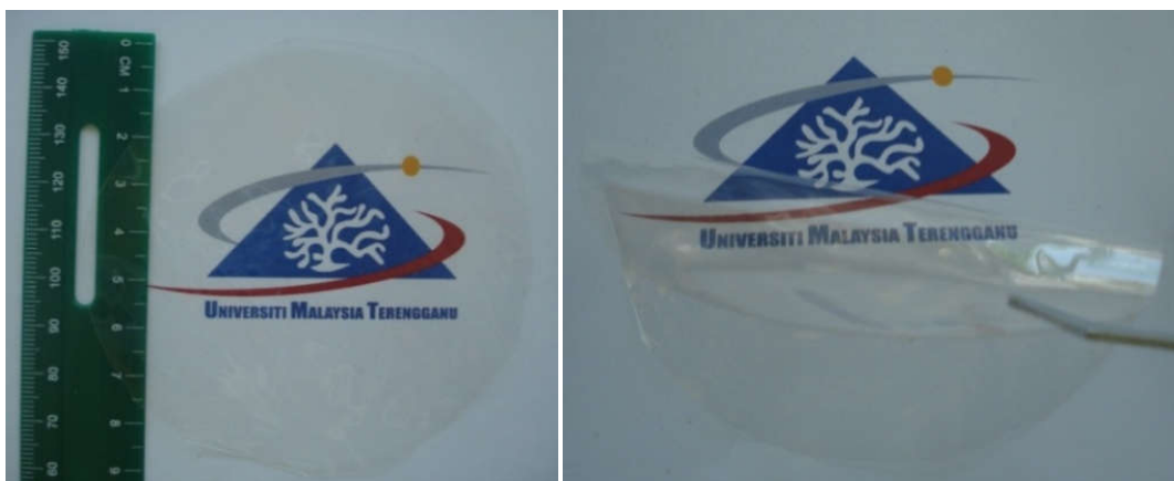
Figure 4.1 A highly translucent and flexible SPE films obtained at room temperature.
