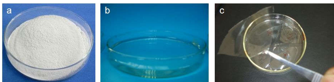
Figure 2.1 The physical appearance of pure CMC, (a) powder, (b) liquid, and (c) solid film.
