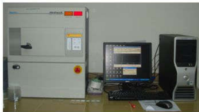
Figure 3.3 The MiniFlex II Rigaku X-ray diffraction spectrometer used in this study.
