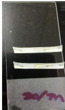
Appendix 11: Thin samples were mounted on a standard microscope slide.
